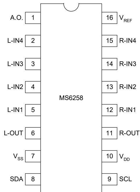
Note: 1. Pin 1 is set to Lo or open , the address code is 88H (10001000B).
