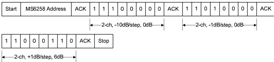
Note: We suggest the gain is set as the power is up. For example, set and fix the gain +10dB, the volume range will be controlled from +10dB to -69dB.
