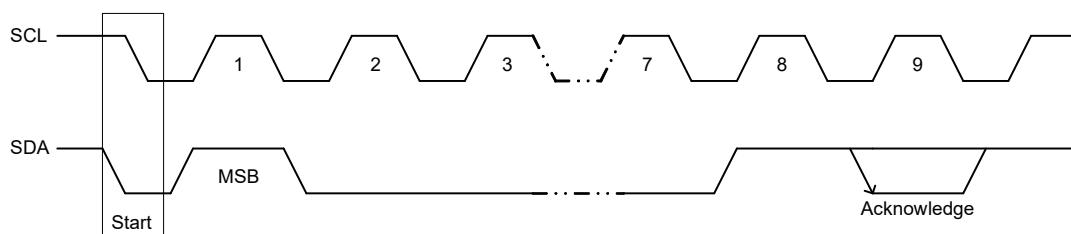
The audio processor that has been addressed has to generate an Acknowledge after receiving each byte, otherwise, the SDA line will remain at the HIGH level during the ninth (9<sup>th</sup>) clock pulse. In this case, the master transmitter can generate the STOP information in order to abort the transfer.
