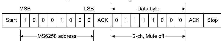
Set gain of 2 channel at 0dB, and selected stereo 1 input.
