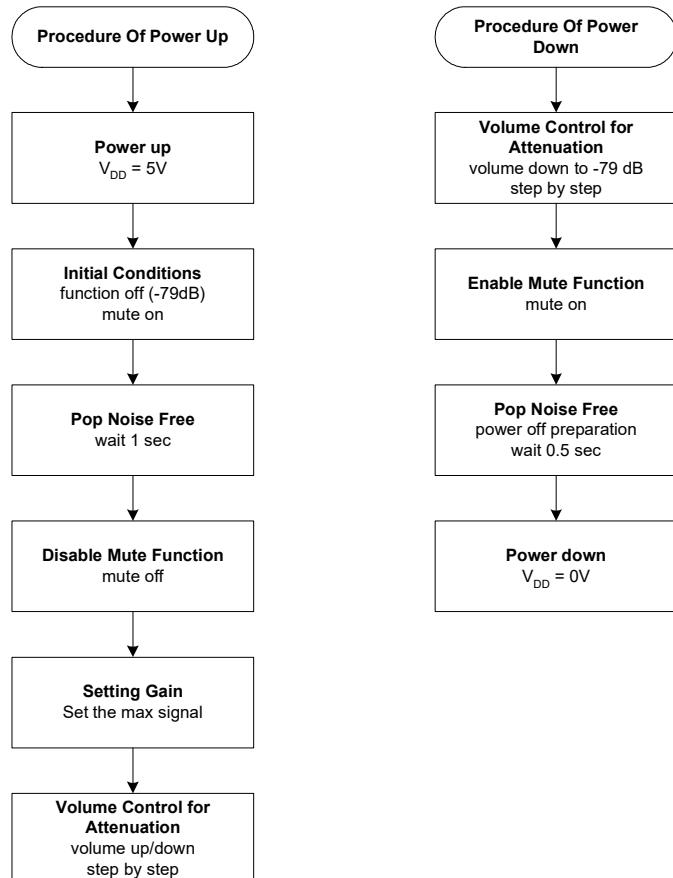
1. The initial condition is -79dB, gain 0dB and mute on when power on.
