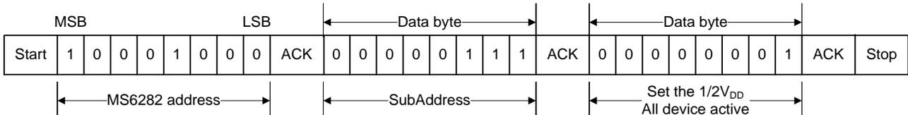
Set Input gain of both channels at +4dB
