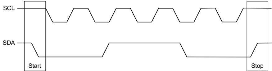
SCL : Serial Clock Line, SDA : Serial Data Line
