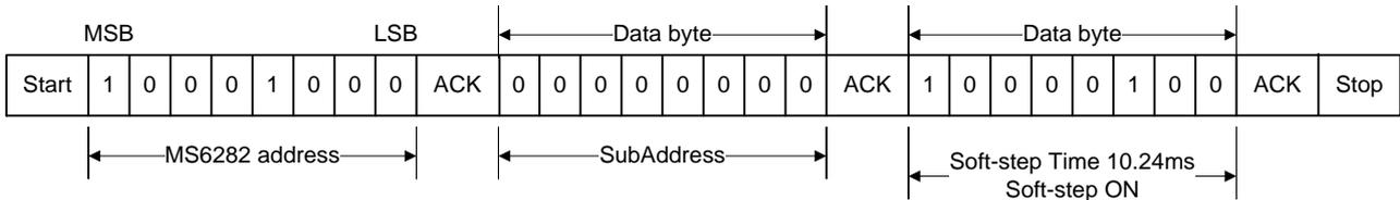
Set the  $1/2V_{DD}$  , All device active.
